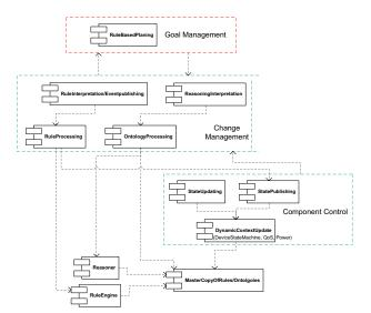
Fig. 1. Architecture of the self-management in Hydra
