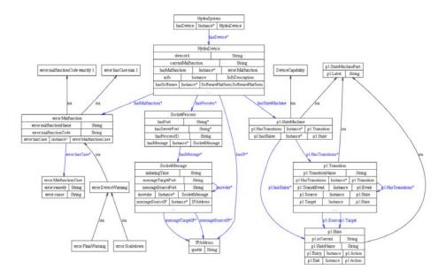
Fig. 3. Partial details of the Diagnosis Manager used ontologies
